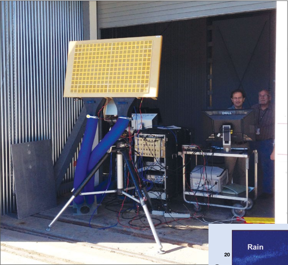
The two-panel prototype MPAR array (left) is used at Hanscom Field to collect observations of aircraft and weather in the vicinity. The range-Doppler plot below is of the weather and aircraft observed by this prototype array.
