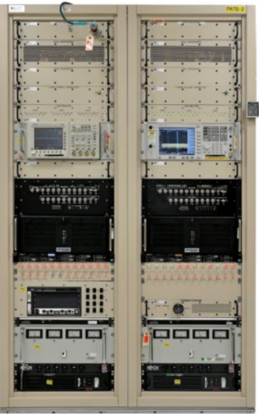
The Over-the-Air Ka-band Test Terminal (far left) and the Protected Tactical System Advanced Test Set (left) will be utilized together to test the new Protected Tactical Waveform. The Lincoln Laboratory–built implementation of the waveform will be used in lab and over-the-air tests to validate the capabilities of vendor implementations of the waveform.
