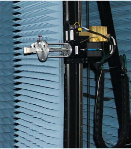
The near-field measurement range at the RF System Test Facility is used to characterize millimeter-wave imaging through common materials and to investigate sparse aperture sampling. Shown above are the near-field probes used for transmitting and receiving millimeter test signals.
