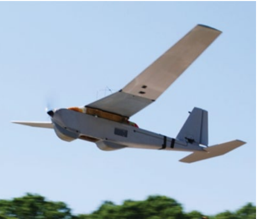
This Puma unmanned aerial vehicle is equipped with the vector sensor that the Laboratory developed to provide a tactical geolocation capability. The Puma's first flight occurred at the Camp Edwards air field in Massachusetts.
