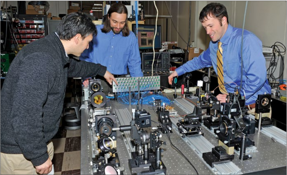
Juan Montoya, Andrew Benedick, and Scot Shaw use prototype technology to demonstrate a new optical phased array beam-combining approach developed at Lincoln Laboratory with support from the Defense Advanced Research Projects Agency (DARPA).
