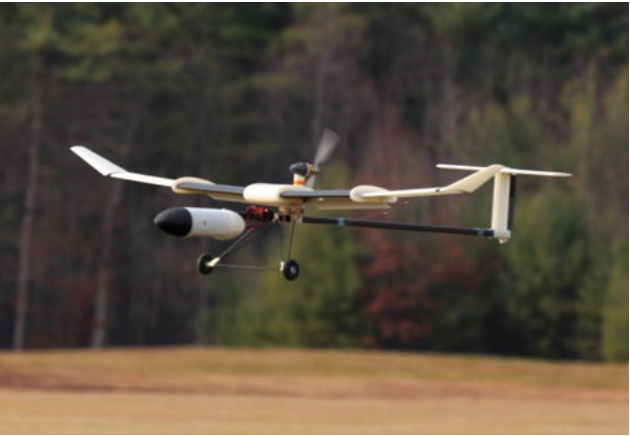
Two Lincoln Laboratory researchers received a distinguished paper award from the Society of Manufacturing Engineers (SME) for their paper on the 3D-printed, extendable-wing Variable Airspeed Telescoping Additive Unmanned Air Vehicle (pictured above). This award, presented at SME’s annual Rapid Prototyping Conference, recognizes a paper that has had a significant impact on rapid prototyping or additive manufacturing.
