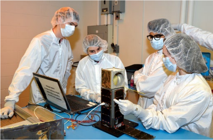
MIT graduate students conduct a final verification of attitude-determination sensors for the Micro-sized Microwave Atmospheric Satellite (MicroMAS) in Lincoln Laboratory’s Environmental Test Laboratory. The MicroMAS project was a collaboration between technical groups within the Laboratory’s Engineering and Space Control mission areas and researchers at MIT’s Space Systems Laboratory to design and build a low-cost nanosatellite capable of providing observations of storm dynamics.
