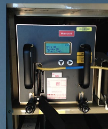
ACAS X logic is implemented in the Honeywell International Inc. prototype used in the 2013 proof-of-concept flight test.
